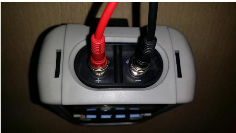
[Insert Test Probe]
